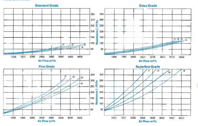
**NOTE:** Initial Resistance/Flow Rate – For 610 × 610 mm Filter
