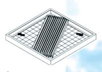
2. Grasp the three outer most pleats on one side of the element and pull to the inner edge of the frame. Repeat process on opposite side.
