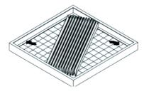
Compress element and place diagonally in holding frame.
