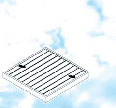
**3.** Compress the two outer most pleats of the element into the inner edges of the frame. Space remaining individual pleats evenly along the face of the frame for best results.
