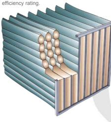
Interpocket filters are extended surface, high capacity air filters. They are designed to provide a cost effective means of handling large air volumes of constant air flow, with high-particulate concentration of sub-micron particles. The media construction combines a compact design with excellent airflow characteristics, providing potential for significant energy savings.
